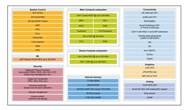
View additional information for i.MX RT700 Crossover MCU with Arm® Cortex®-M33, NPU, DSP and GPU Cores.
