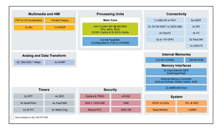
View additional information for i.MX RT1040 Crossover MCU with Arm® Cortex®-M7 Core Operating Up to 600 MHz and Extended Temperature Range.
