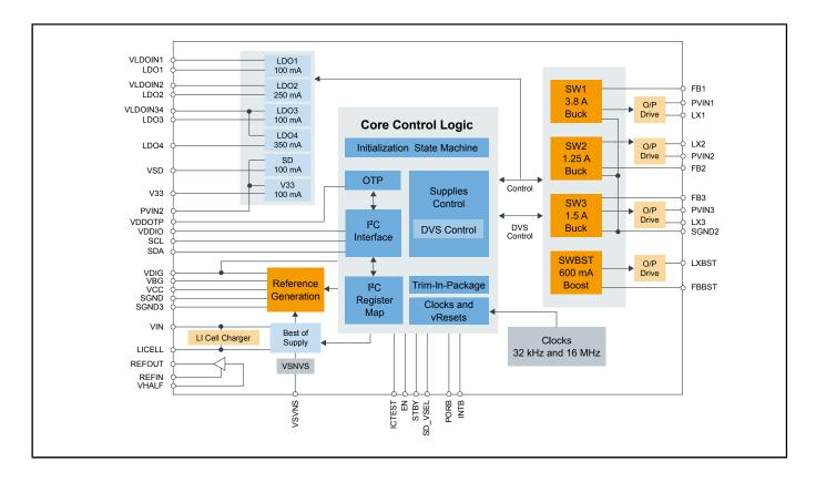
View additional information for Multi-Output DC-DC Regulator for Low Power LS1 Communication Processors.
