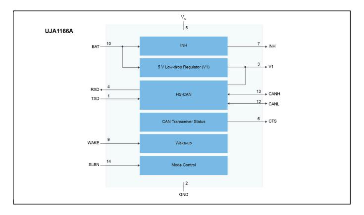
View additional information for High-Speed CAN Transceiver with 5 V LDO and Sleep Mode.
