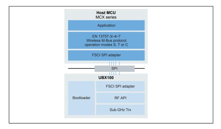
View additional information for UBX100 Sub-GHz Wireless M-Bus Solution.
