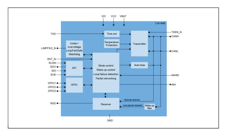
View additional information for CAN SIC Transceiver with Partial Networking and Advanced System Monitoring, CAN FD Data Rates Up to 8 Mbit/s.
