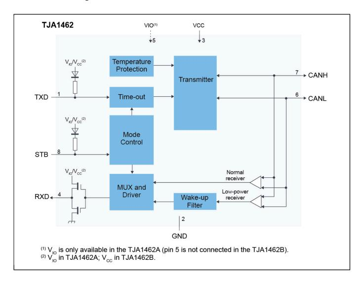
View additional information for CAN Signal Improvement Capability Transceiver with Standby Mode.
