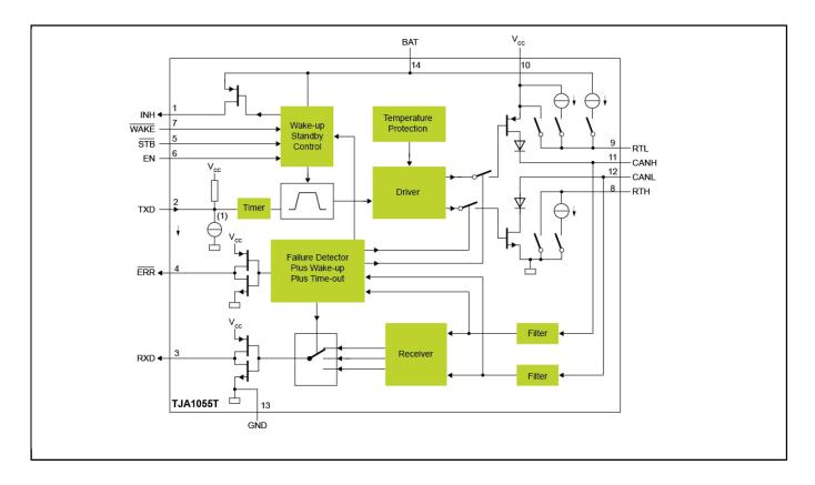
View additional information for Fault-Tolerant CAN Transceiver.
