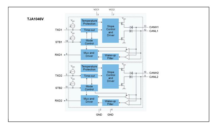
View additional information for VeLIO Certified, Dual High-Speed CAN Transceivers with Standby Mode for Automotive Applications.
