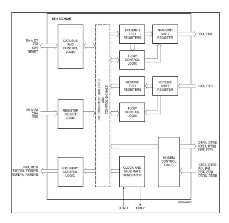
View additional information for 5 V, 2.2 V and 2.5 V dual UART, 5 Mbit/s (max.), with 64-byte FIFOs.
