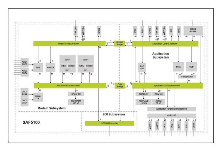
View additional information for Software Defined Radio Processor for V2X Communication.
