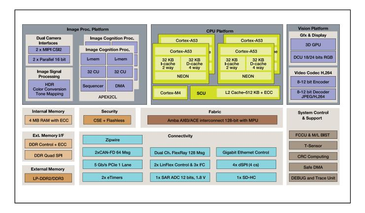
View additional information for S32V2 Processors for Vision, Machine Learning and Sensor Fusion.
