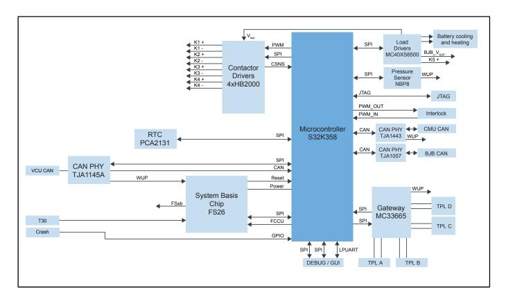
View additional information for S32K358 Battery Management Unit (BMU) for High Voltage Battery Management System (HVBMS) Reference Design Board.
