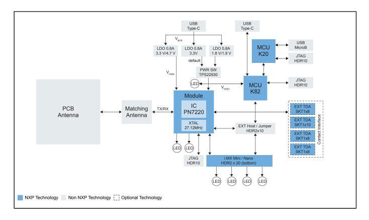
View additional information for Development Board for PN7220 NFC Controller with Two Host Configuration.
