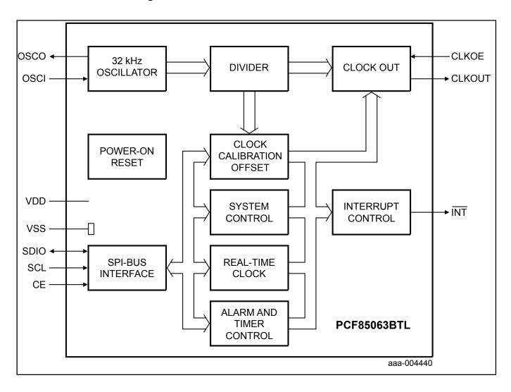
View additional information for Tiny Real-Time Clock/Calendar with Alarm Function and SPI-Bus.
