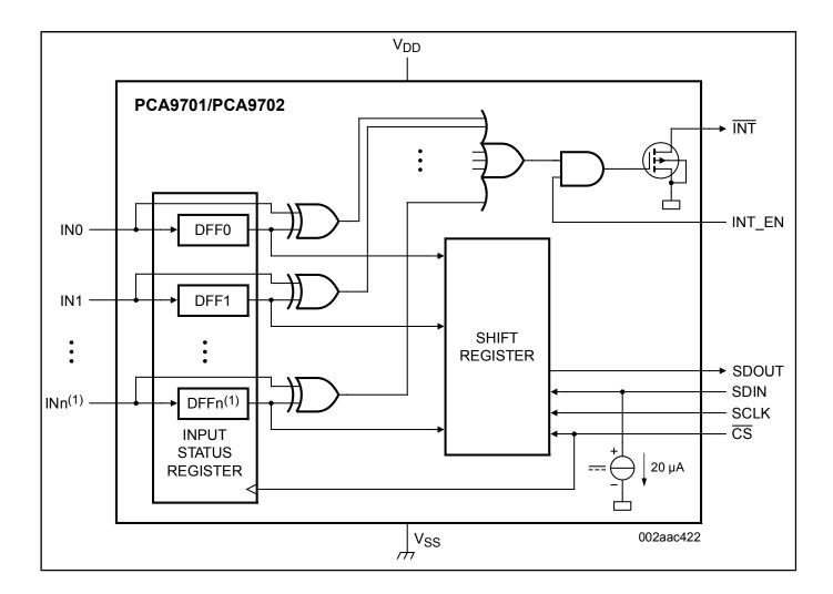
View additional information for 18 V Tolerant SPI 16-Bit/8-Bit GPI with INT.
