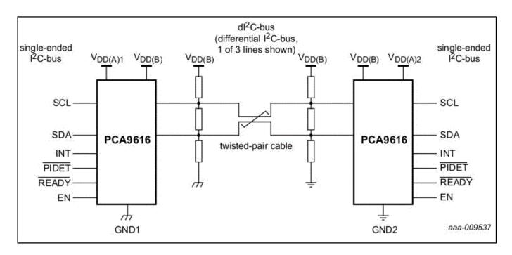
View additional information for Three-Channel Multipoint Fast-Mode Plus Differential I<sup>2</sup>C-Bus Buffer with Hot-Swap Logic.
