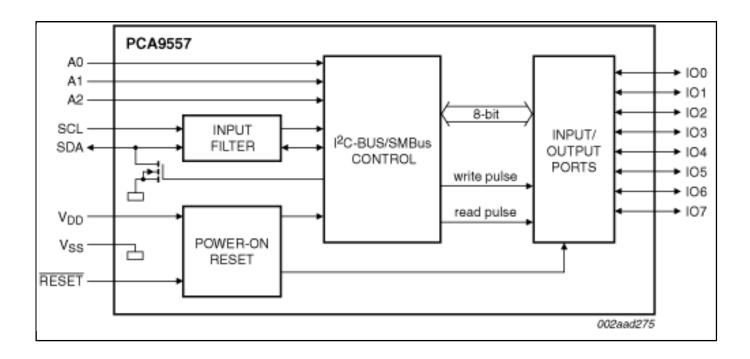
View additional information for 8-Bit I<sup>2</sup>C-Bus and SMBus I/O Port with Reset.
