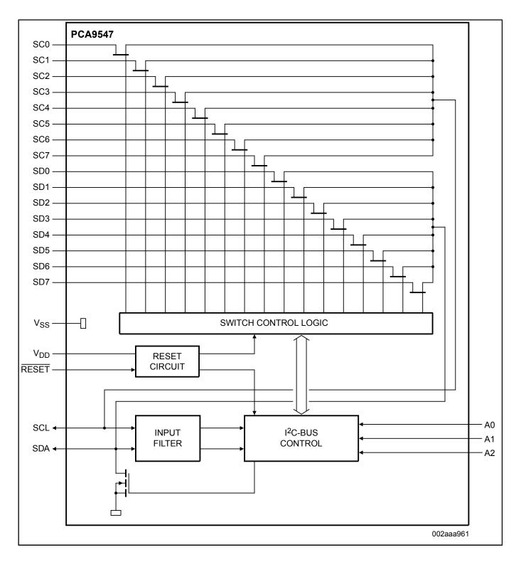
PCA9547BS, PCA9547D, PCA9547PW Block Diagram
