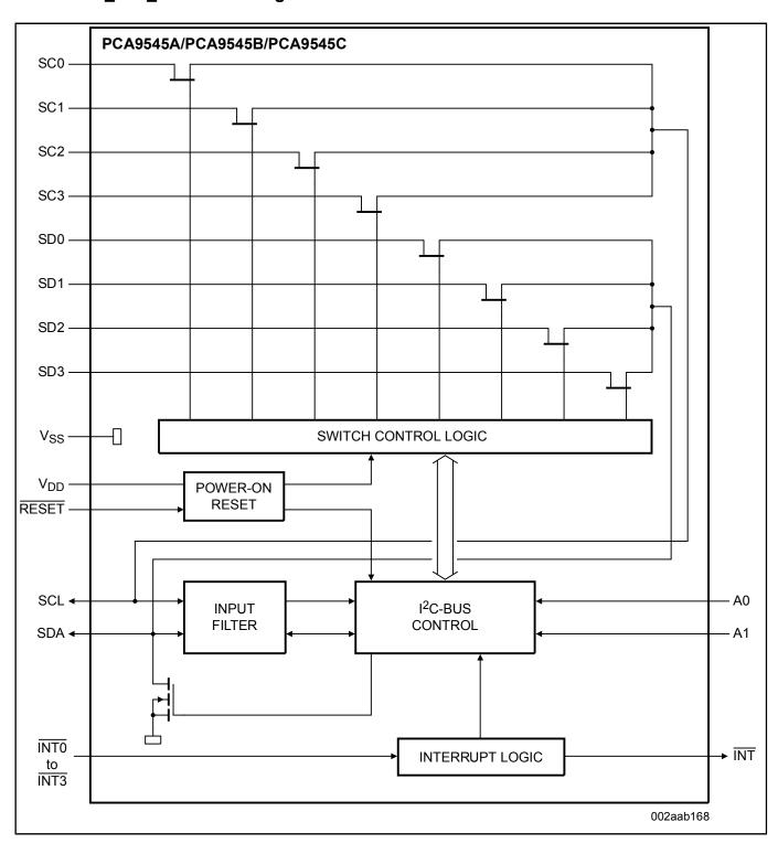
View additional information for Four-Channel I2C-Bus Switch with Interrupt Logic and Reset.
