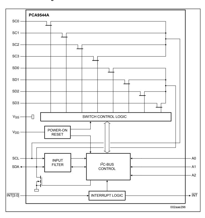
PCA9544ABS, PCA9544AD, PCA9544APW Block Diagram
