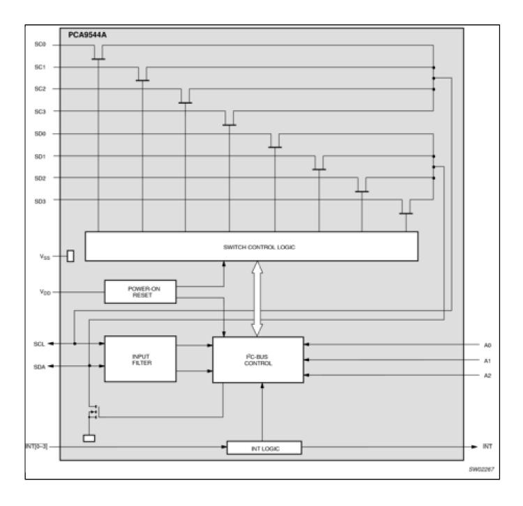
View additional information for Four-Channel I<sup>2</sup>C-Bus Multiplexer with Interrupt Logic.
