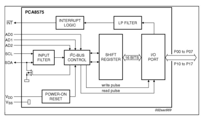
View additional information for Remote 16-Bit I/O Expander for I<sup>2</sup>C-Bus with Interrupt.
