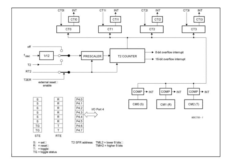
Block diagram: P80C562EBA Block Diagram
