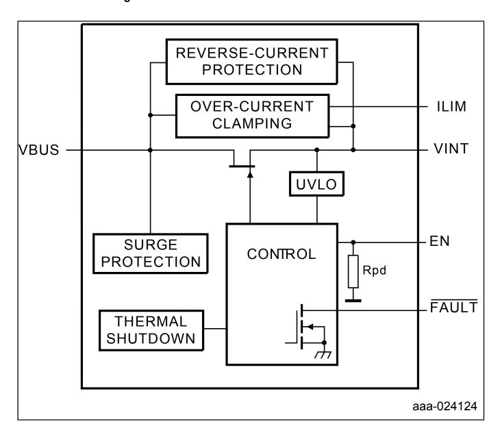
View additional information for USB PD and Type-C Current-Limited Power Switch.
