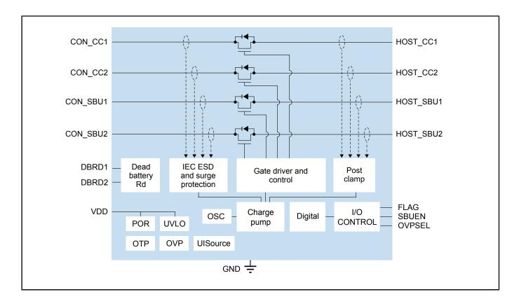
View additional information for 48 V Type-C CC and SBU Protection IC for USB PD3.1 EPR.
