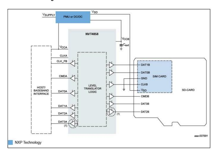
View additional information for SD, SDIO, Mini SD, Micro SD and SIM Card Voltage Level Translator with EMI Filter and ESD Protection.
