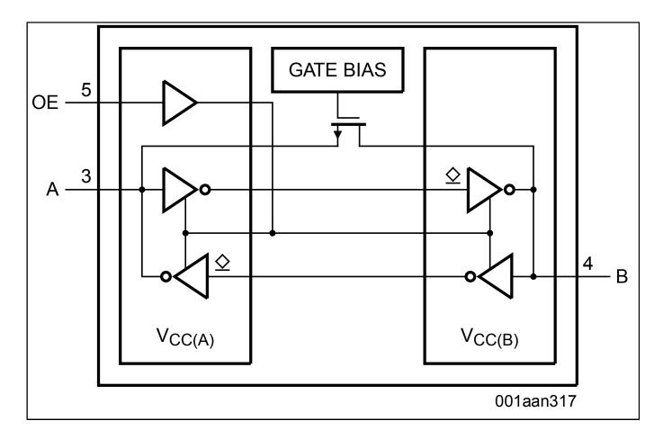
View additional information for Dual-Supply Translating Transceiver (Open-Drain, Auto-Direction Sensing).
