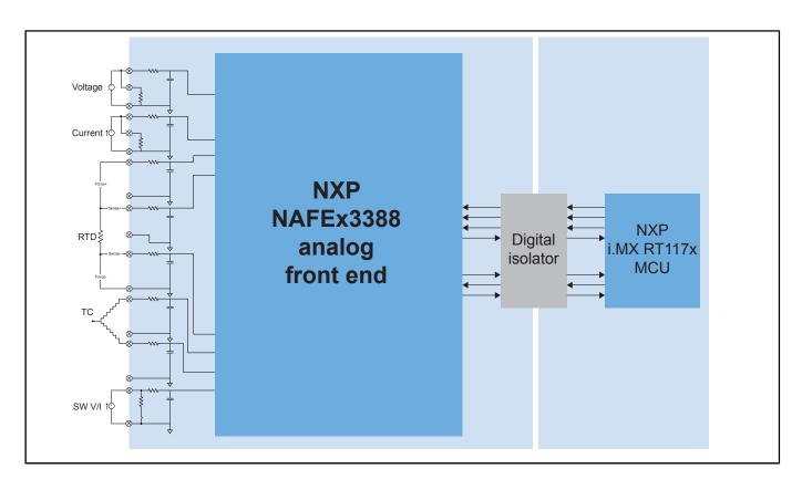
View additional information for Highly Configurable 8/4 Channel 24/16 bits ±25 V Universal Input Analog Front-End with Excitation Sources.
