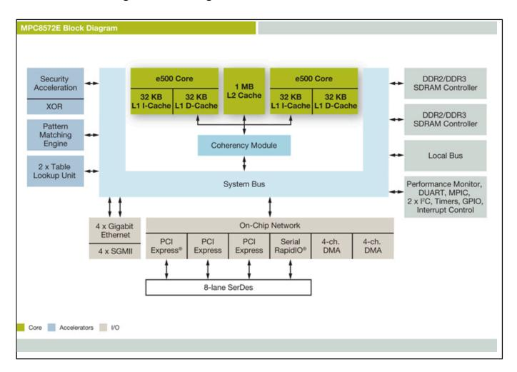
View additional information for PowerQUICC® III Processor with DDR2/3, Pattern Matching Engine, PCI Express®.
