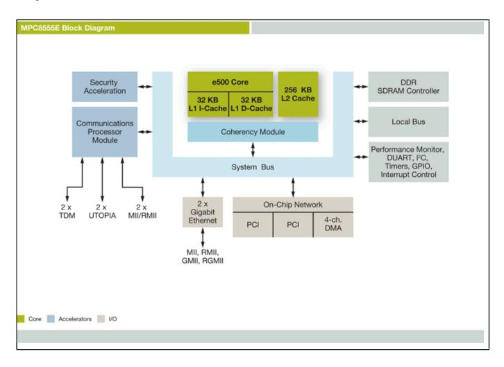
View additional information for PowerQUICC® III Processor with TDM, DDR, PCI, 1 GB Ethernet, Security, CPM with UTOPIA.
