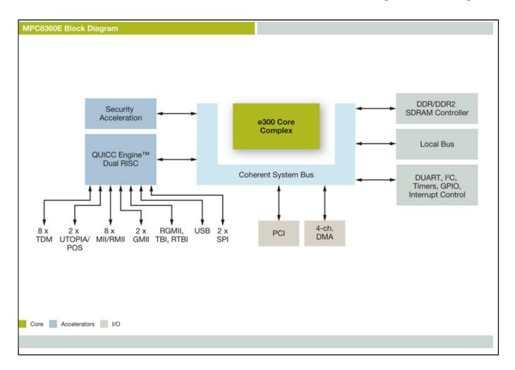
View additional information for PowerQUICC® II Pro Processor with DDR2, TDM, PCI, Security, USB, QUICC Engine® with 1 GB Ethernet, UTOPIA.
