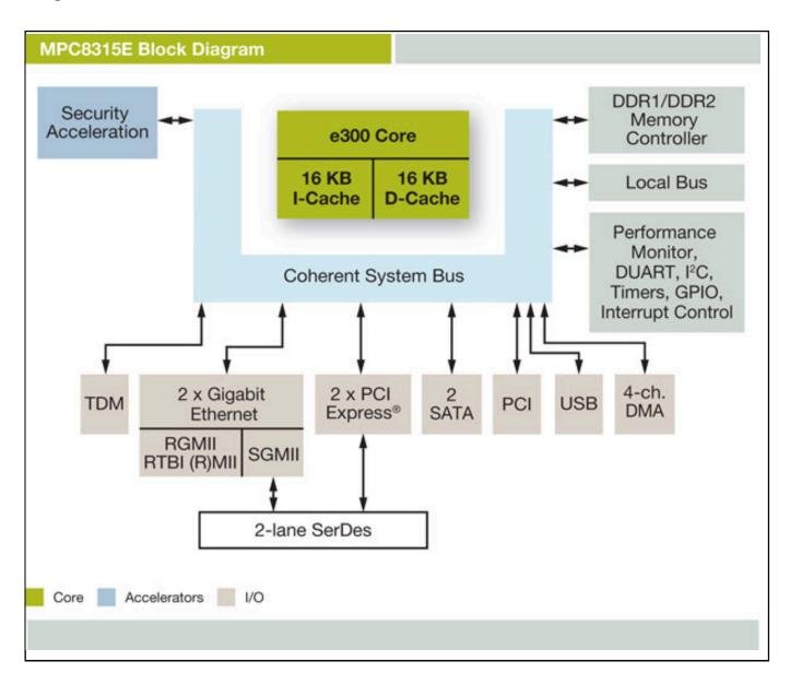
View additional information for Low-Power PowerQUICC® II Pro Processor with DDR2, TDM, PCI, PCI Express, SATA, 1 GB Ethernet, Security, USB.
