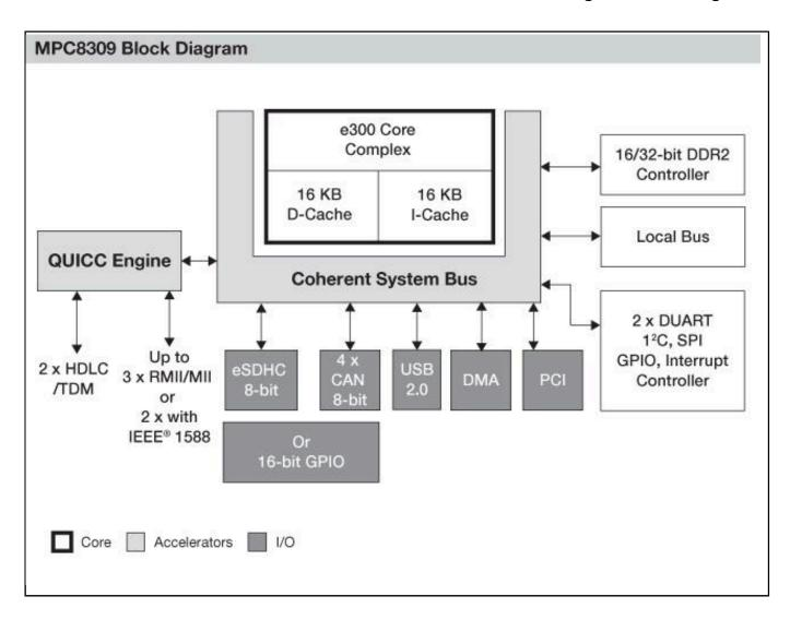
NXP PowerQUIICC MPC8309 Communications Processor Block Diagram Block Diagram
