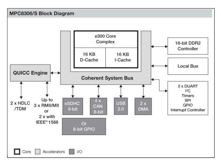
View additional information for Low-Power PowerQUICC® II Pro Processor with DDR2, eSDHC, 128-ch. HDLC/TDM, 10/100 Ethernet, USB, IEEE® 1588.
