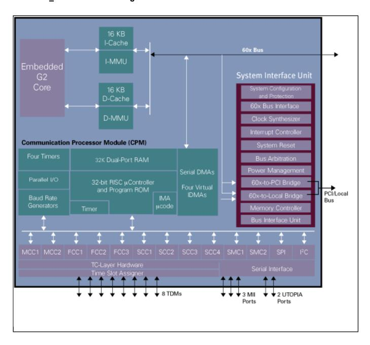
View additional information for PowerQUICC® II Processor with PCI, 256-ch. HDLC, UTOPIA II, 10/100 Ethernet, IMA.
