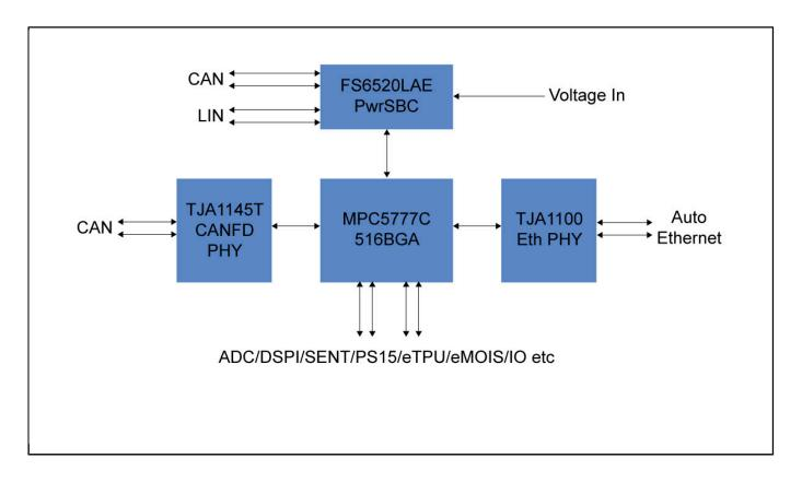
View additional information for MPC5777C BMS and Engine Control Development Board.
