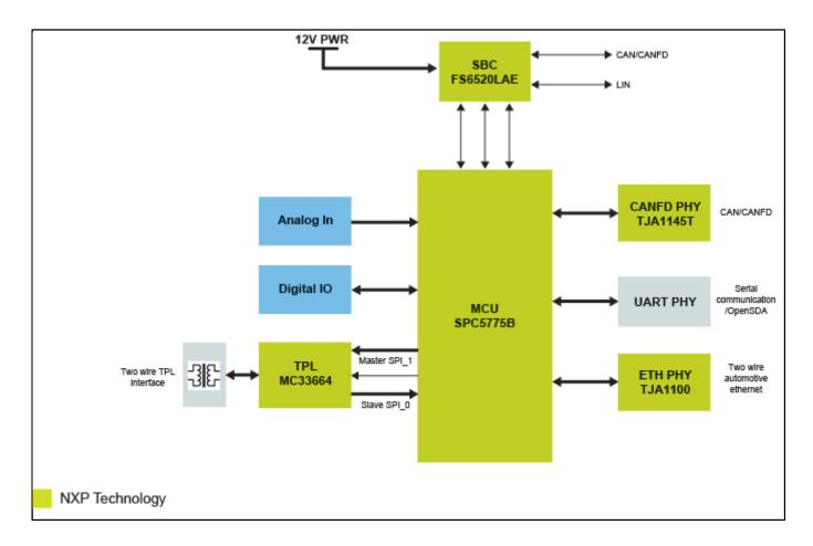
MPC5775E-EVB development board architecture Block Diagram
