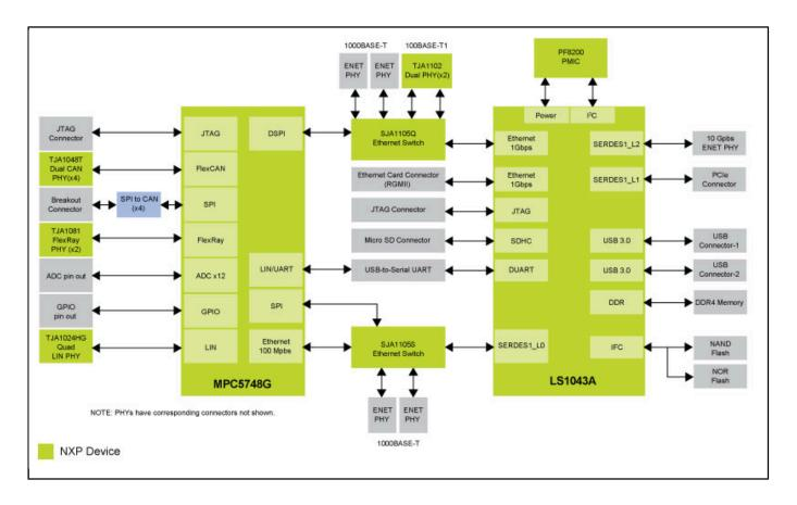
View additional information for MPC-LS Vehicle Network Processing Evaluation Board.
