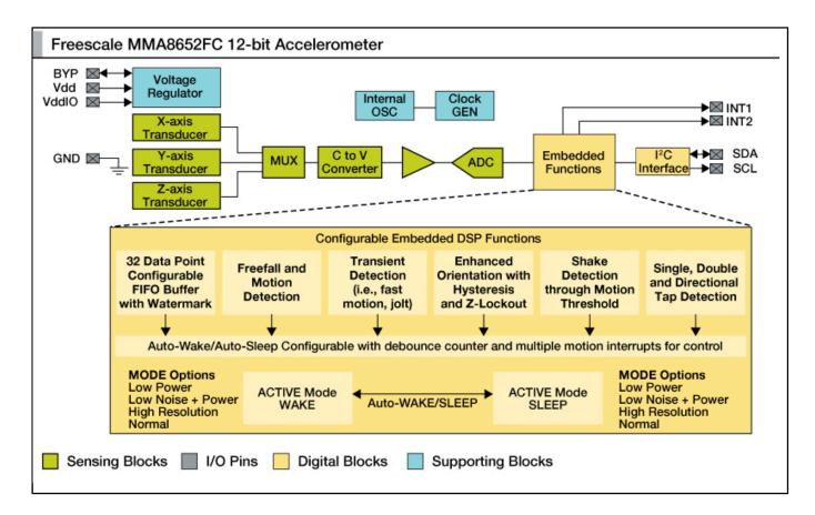
View additional information for ±2g/±4g/±8g, Low g, 12-Bit Digital Accelerometer.
