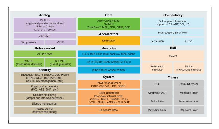
View additional information for MCX N23x Highly Integrated MCUs with On-Chip Accelerators, Intelligent Peripherals and Advanced Security.
