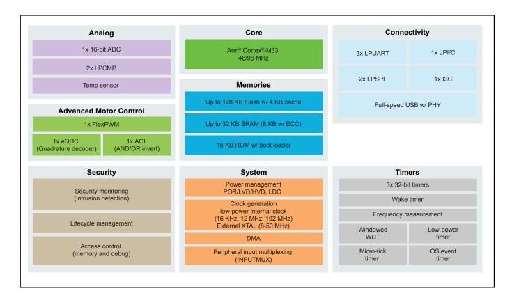
MCX A144/5/6, A154/5/6 Block Diagram Block Diagram
