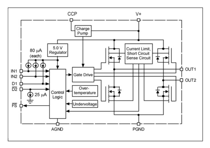
H-Bridge, Brushed DC Motor Driver, 5-28V, 5A, 10kHz Block Diagram
