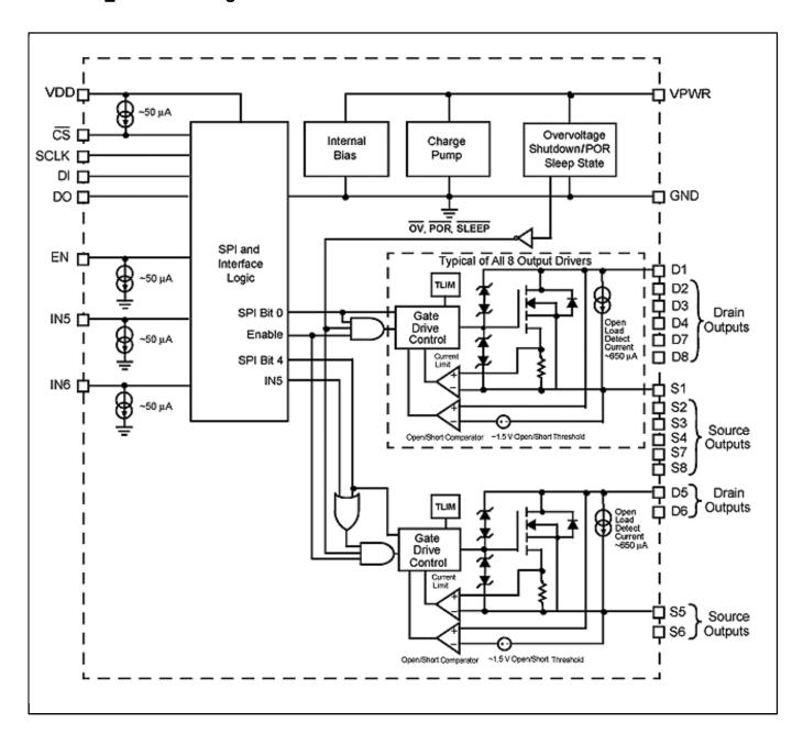
View additional information for Octal Serial Switch with SPI.
