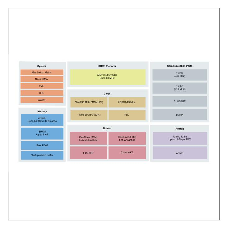
View additional information for LPC860: 32-Bit Arm® Cortex®-M0+-Based Low-Cost MCU with I3C Interface.
