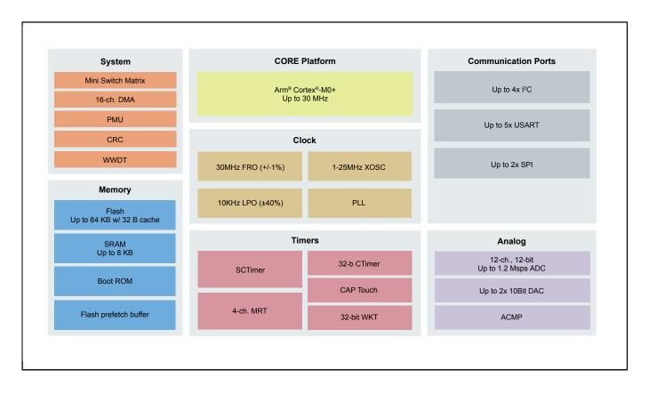
View additional information for LPC840: 32-Bit Arm® Cortex®-M0+-Based Low-Cost MCU.
