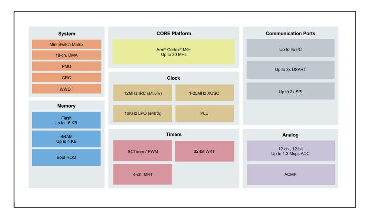
View additional information for LPC820: 32-Bit Arm® Cortex®M0+-Based Low-Cost MCU.
