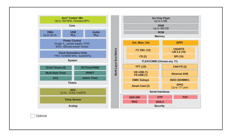
View additional information for Power-Efficient Microcontrollers (MCUs) with Advanced Peripherals Based on Arm® Cortex®-M4 Core.
