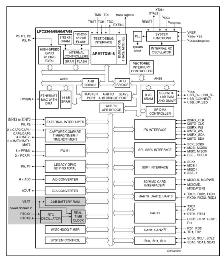
View additional information for Arm7<sup>™</sup> with 512 kB flash, 58 kB SRAM, Ethernet and 10-bit ADC.
