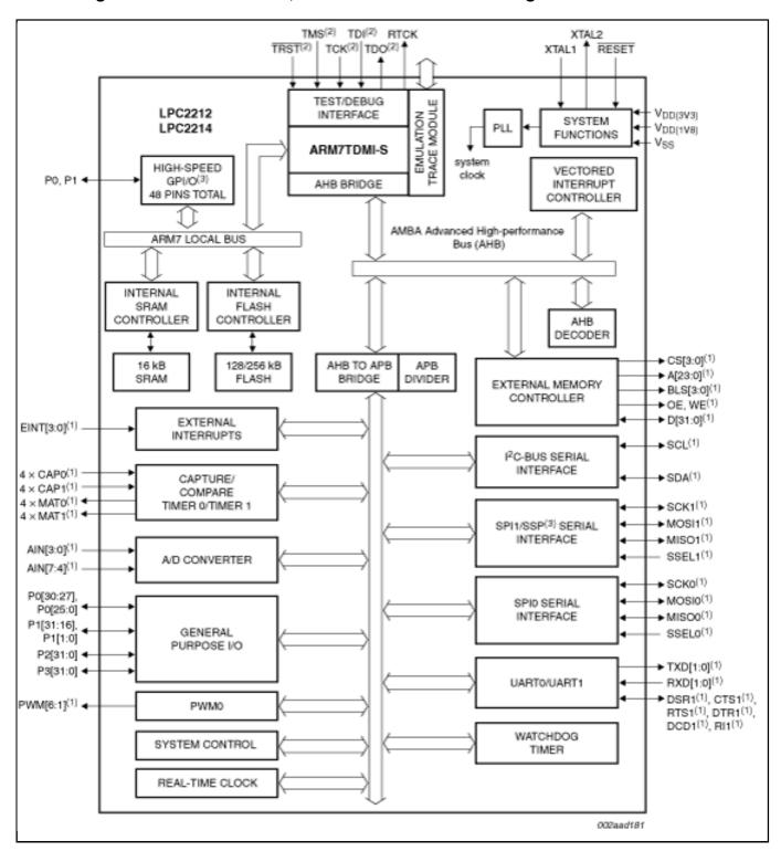
View additional information for Single-chip 16/32-bit Arm® microcontrollers; 128/256 kB ISP/IAP flash with 10-bit ADC and external memory interface.
