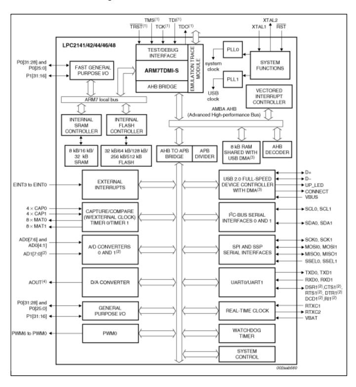
View additional information for Single-chip 16-bit/32-bit microcontrollers; up to 512 kB flash with ISP/IAP, USB 2.0 full-speed device, 10-bit ADC and DAC.
